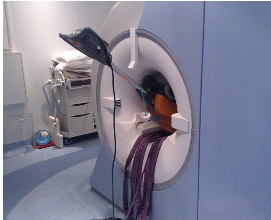
MRI accident on a 1.5T MR system. A floor polishing machine was attracted by the magnetic field. It could only be removed by ramping down the magnetic field. Shown is the back side (head end) of the MRI. Reproduced from: https://commons.wikimedia.org/wiki/File:MRI_accident_on_a_1.5_Tesla_MR_system.jpg
