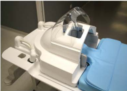
Head coil (32 channels)
